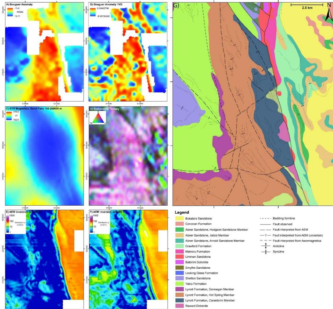
**Figure 3. a) Bouguer anomaly; b) 1<sup>st</sup> Vertical derivative of the Bouguer anomaly; c) Reduced to pole magnetics, band pass filtered 180-25 000 m; d) Ternary plot of Radiometrics; e) AEM inversion depth slice at 200-250 m; f) AEM inversion depth slice at 350-400 m; g) Geological interpretation**
