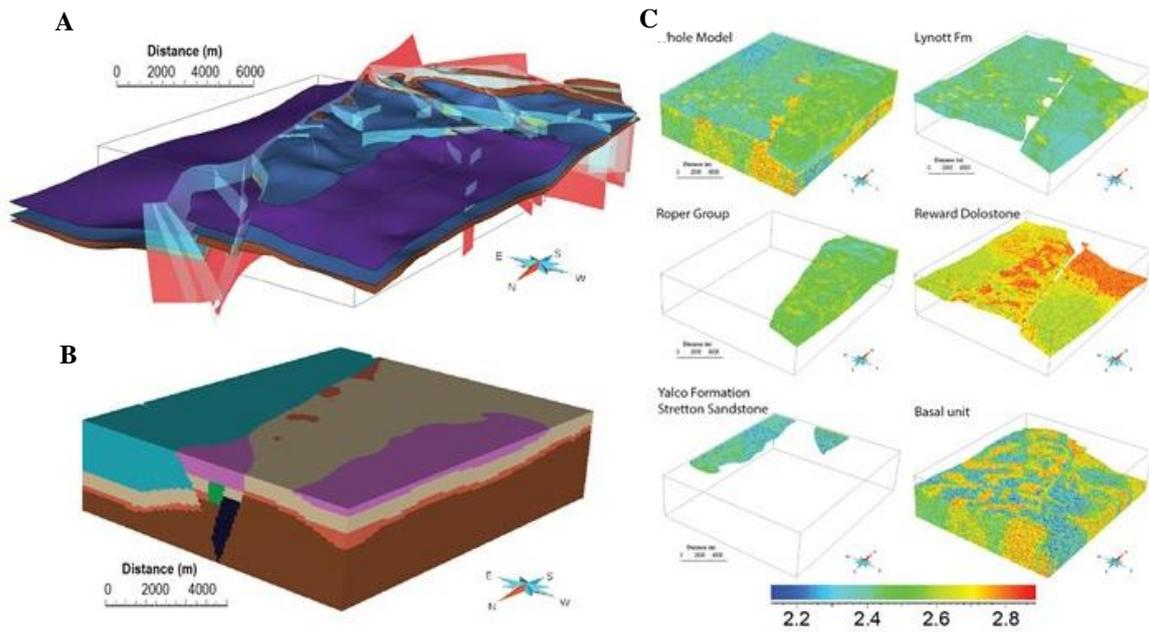
Figure 4. a) Initial geological model; b) Volume of interest for inversion; c) Density distribution within each model region.
