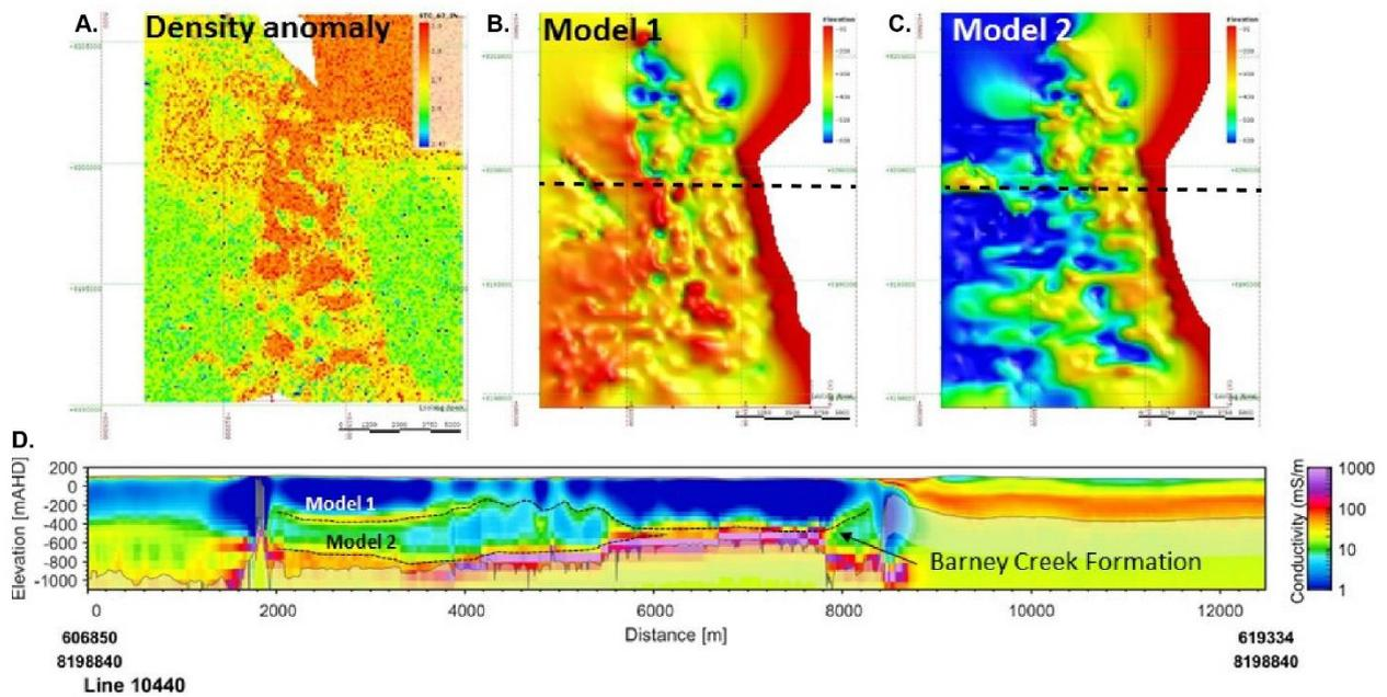
Figure 5. a) Depth slice of density anomaly from gravity inversions. Interpretation of depth to Barney Creek formation from VTEM data in b) model 1; and c) model 2; d) Section of 1D VTEM inversion showing two conductive anomalies interpreted to produce models 1 and 2 (section location shown in b and c).
